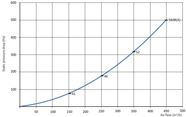
Static pressure drop is measured in accordance with ISO standard 5167-1. Noise level is measured in accordance with ISO standard 3743. Indicated sound level refers to sound pressure level.
