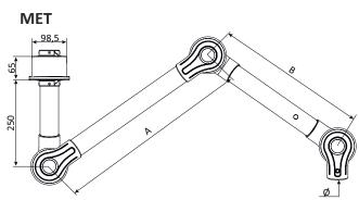
MET for ceiling mounting, excluding ceiling bracket MTI. MEV for wall mounting, including wall bracket MVK.
