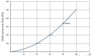
Static pressure drop is measured in accordance with ISO standard 5167-1. Air flow (m<sup>3</sup>/h) Noise level is measured in accordance with ISO standard 3743. Indicated sound level refers to sound pressure level.
