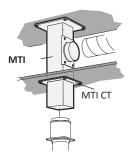
The ceiling bracket functions as a simple and stable duct for outgoing air, avoiding the need for expensive ducting and additional holes through false ceilings. On request, the MTI can be supplied in lengths exceeding 2 m.
