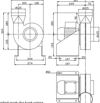
VSB14 **default motor configuration** is 0.18kw/4-pole/1-phase supplied ready for hard-wiring. All VSB Series Fans incorporate a 20mm drain fitted at the lowest point in the case.
