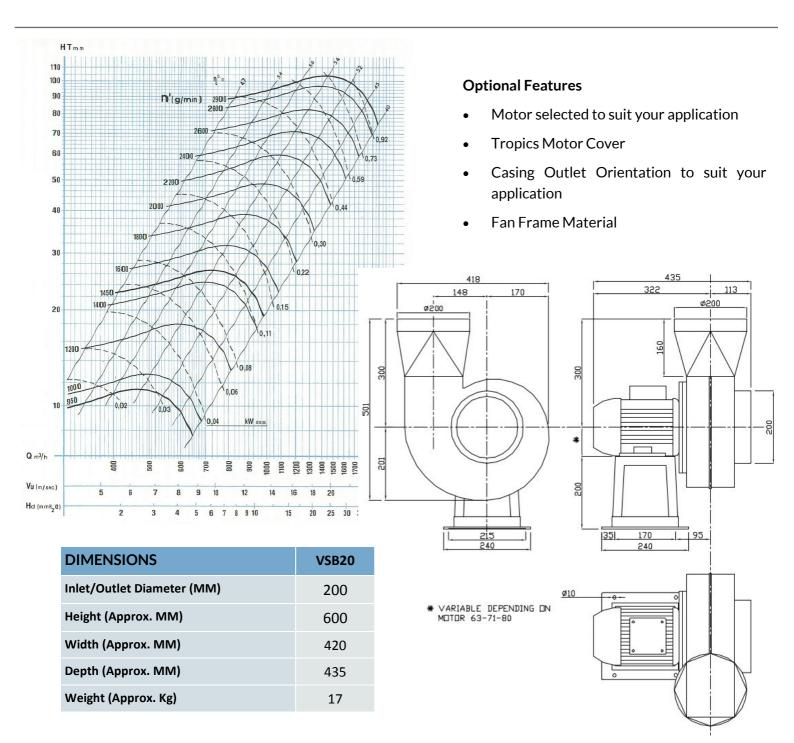
VSB20 **default motor configuration** is 0.75kw/4-pole/3-phase supplied wired for 220v DELTA wiring for VSD control.
